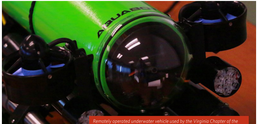
Remotely operated underwater vehicle used by the Virginia Chapter of the Nature Conservancy and the Virginia Institute of Marine Science to assess water quality benefits of shellfish farms.
